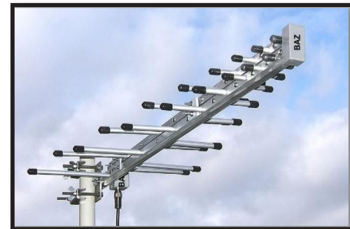
Figure 3b. Typical Log-Periodic Dipole Antenna [BAZ Antennas 2012]
